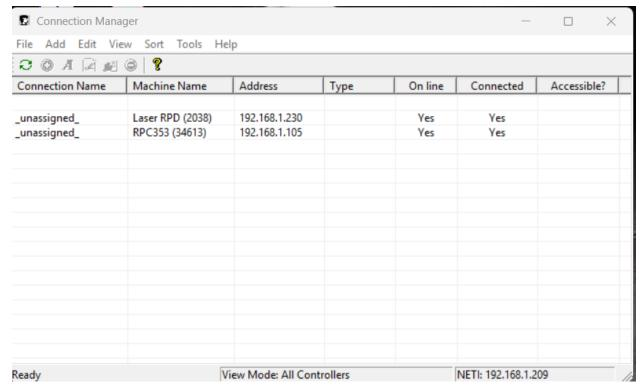
21. This is showing my 2 machines connected, 1 laser and 1 rotary machine.
