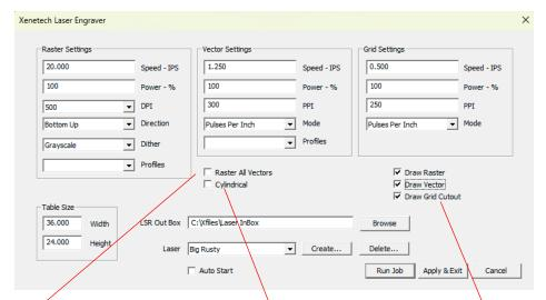
Raster all Vectors allow you to engrave very thin high detail lines for small detail engraving
