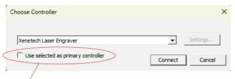
If you are not using any other controllers you can check the "Use selected as primary controller" box to eliminate this step going forward. With this checked this dialog is bypassed and the Xenetech Laser Engraver EDI launches automatically.
